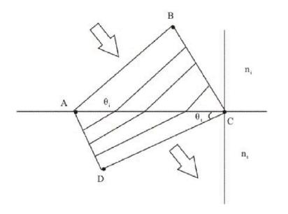
Figure 1: Incident and transmitted plane wavefronts at a flat interface between media with different indices of refraction  $n_i$  and  $n_i$ . The angles of incidence and of refraction are  $\theta_i$  and  $\theta_i$ .
